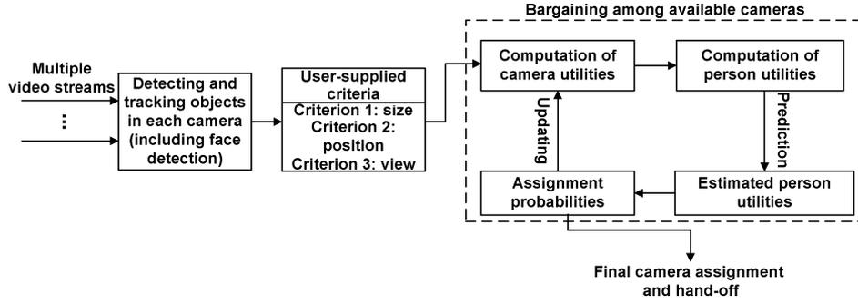
Fig. 1. Game theoretic framework for camera assignment and handoff.
