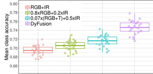
Fig. 4: Mean class accuracy for 54 experiments where random scale, SNR and contrast values are applied to test samples.
