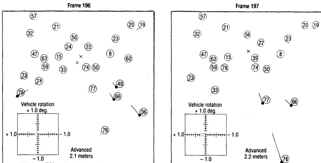
Figure 6. The displacement vectors, the resulting fuzzy FOE (shaded area), camera rotations about two axes, and estimated advancement.
