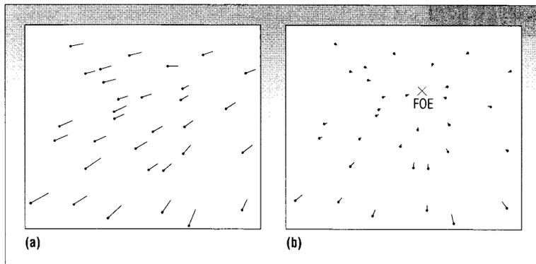
**Figure 1. General-motion field: (a) a typical displacement field obtained from a moving camera undergoing translation and rotation; (b) the displacement field after removing the rotational component of motion. The approximate location of the FOE is marked by a cross.**
