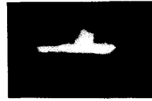
Fig. 7. Segmentation of ship image shown in Fig. 3 by using technique 1.
