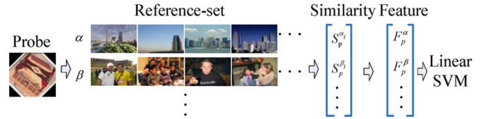
Fig. 2. The flowchart of the reference-based classification scheme.
