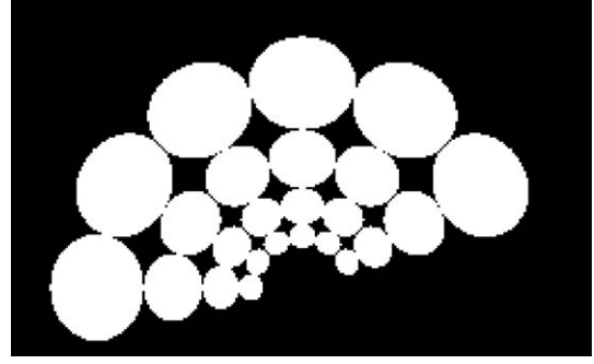
Fig. 3. The filter set in the frequency domain indicates the half-peak magnitude.
