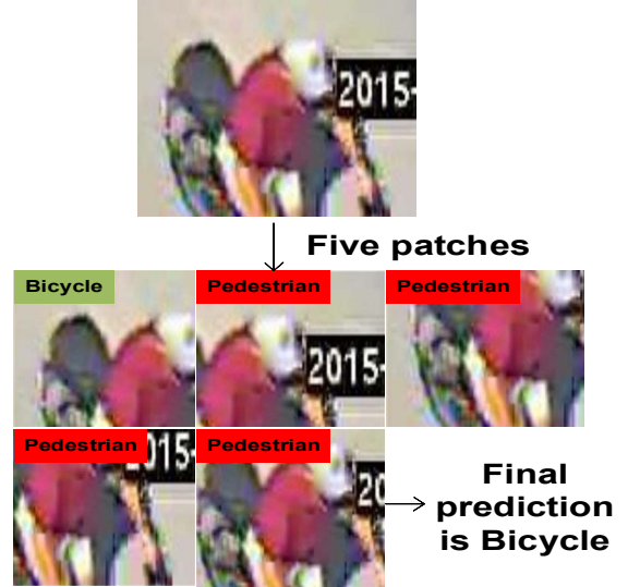
Fig. 6: Network C correctly classifies bicycle that was misclassified as pedestrian by Network B.
