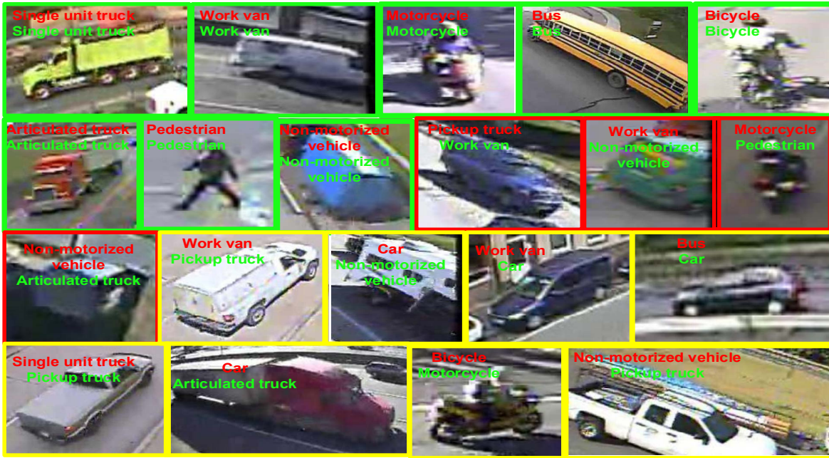
Fig. 6: Classified images from the validation dataset using EDeN. The red text is the ground-truth and the green text is the predicted class. The images in the green frame are correct classification, the images in the red frame are wrong classifications and the images in the yellow frame are noisy data with wrong ground-truth but EDeN predicted them correctly.
