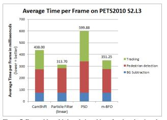
Figure 7. Even with multi-threaded tracking of each pedestrian, the number of pedestrians in the scene (over 40) saturates all available CPU resources (numbers are averaged over 30 runs on an Intel Xeon E5345 2.33GHz quad-core CPU).
