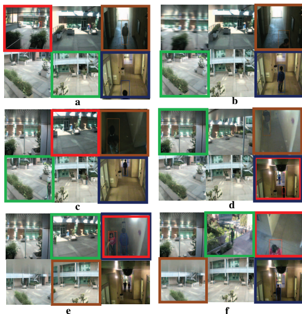
Figure 3: Experimental results in the 6 cameras 4 persons case. Figures are boxed in the same color as the person that they are assigned to follow.
