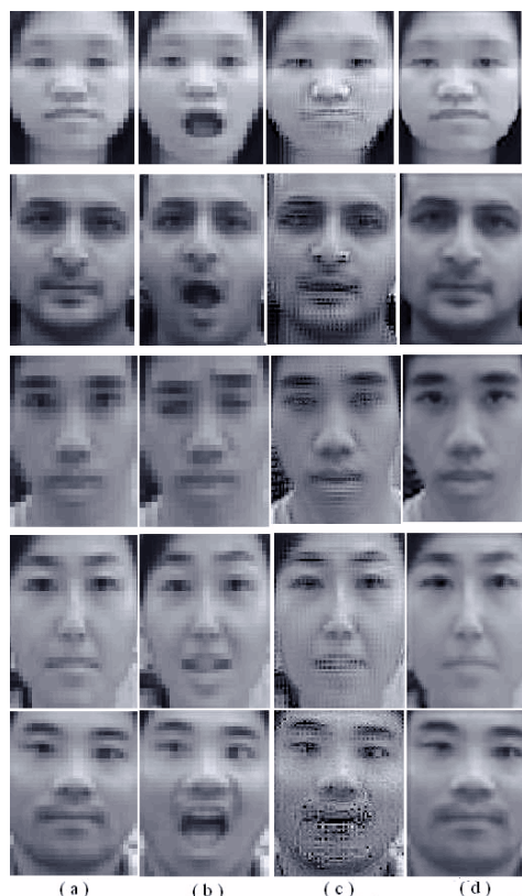
Figure 7. Super-resolution Results. (a)-(b) Low-resolution images. (c)Reconstructed SR images using global registration. (d)Reconstructed SR images using global and our RAIFFD local deformation approach.
