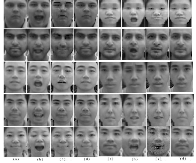
Fig. 3. Super-resolution Results using SR algorithms in [1].(a)-(b) Low-resolution images. (c)Reconstructed SR images using global registration. (d)Reconstructed SR images using global and our RAIFFD local deformation approach.
