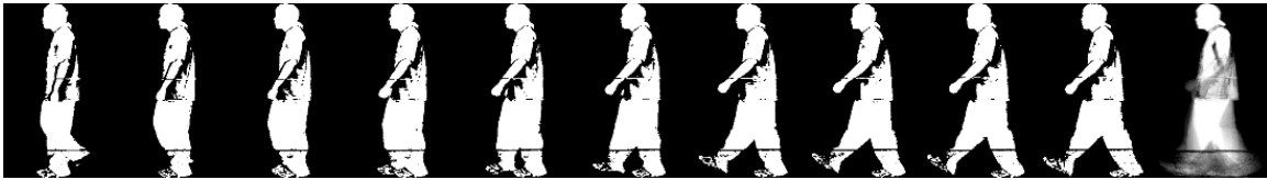
Figure 2. Examples of normalized and aligned silhouette images in a gait cycle. The right most image is the corresponding gait energy image (GEI).
