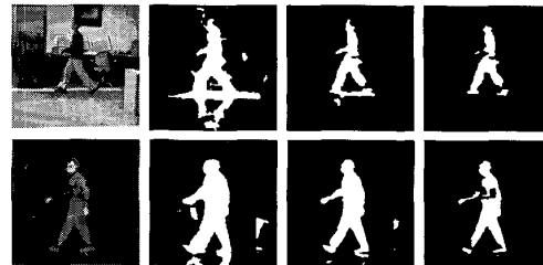
Figure 1. Human silhouette extraction results from color image (top row) and thermal image (bottom row) using background subtraction method with increasing thresholds from left to right (the leftmost image is the original image).
